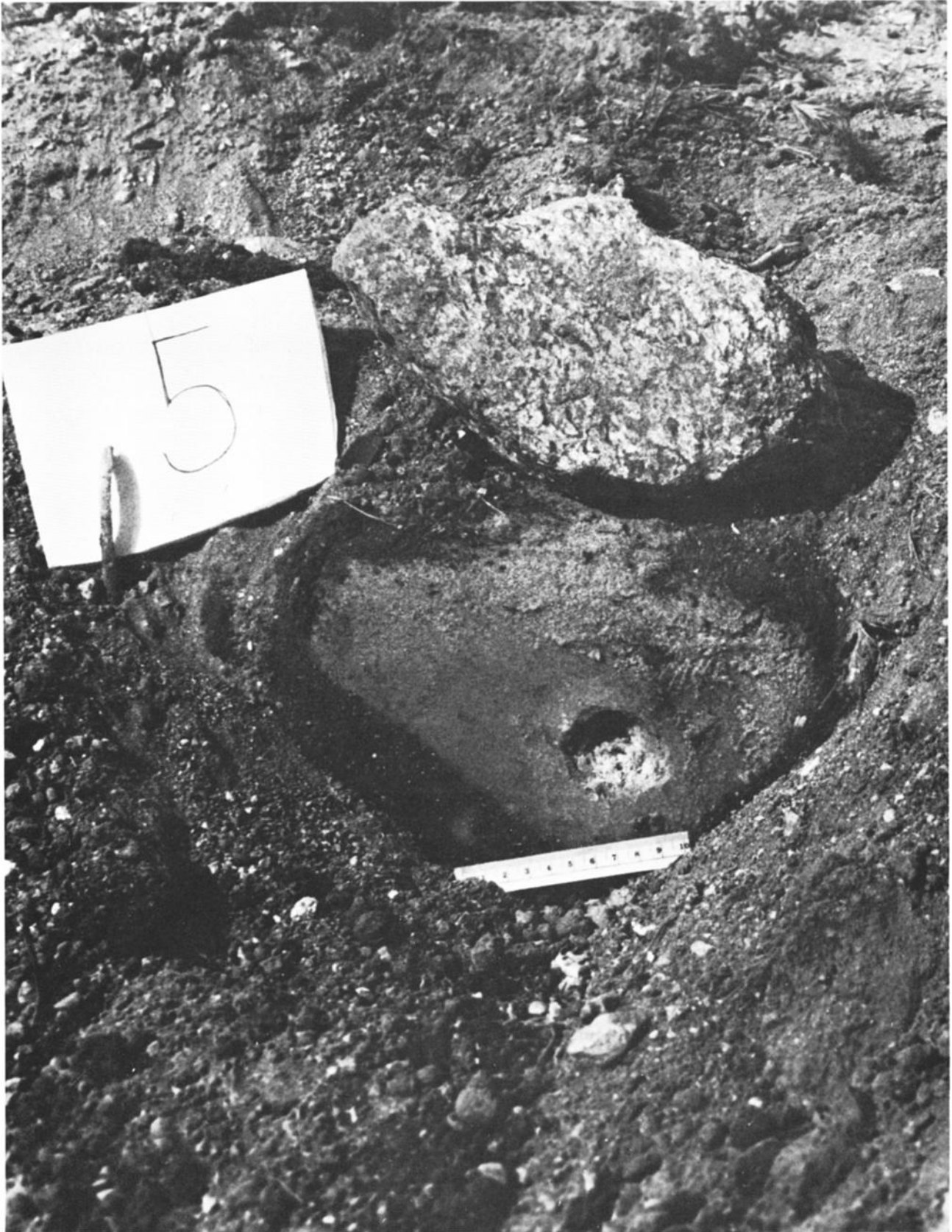
Fig. 1. Crater 5 in ice-saturated sand showing an example of the craters discussed in this report and the target arrangement of ice-saturated sand block bunkered by sand with one vertical face exposed. Note the relatively large depth/diameter ratio ( \sim 0.4 compared to typical hard rock values of \sim 0.2 ) and the system of cracks surrounding the crater to approximately one crater radius beyond the slightly raised rim. White scale bar is \sim 10.5 cm long.
