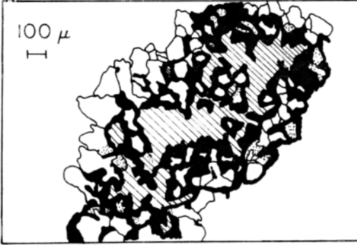
Fig. 11a. Sketch of the typical occurrence of the four different \text{SiO}_2 regions in a class 4 rock: quartz grains (white), opaque rims (black) on many of the quartz grains, and a vesicular glass core (striped) surrounded by the opaque rim. A few symplektic regions (dotted pattern) are shown schematically on the quartz grains.
